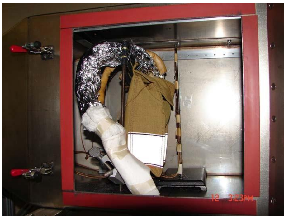
Figure 4 Pocket inside FEE for testing. Radio is inside with insulated cable attached.
