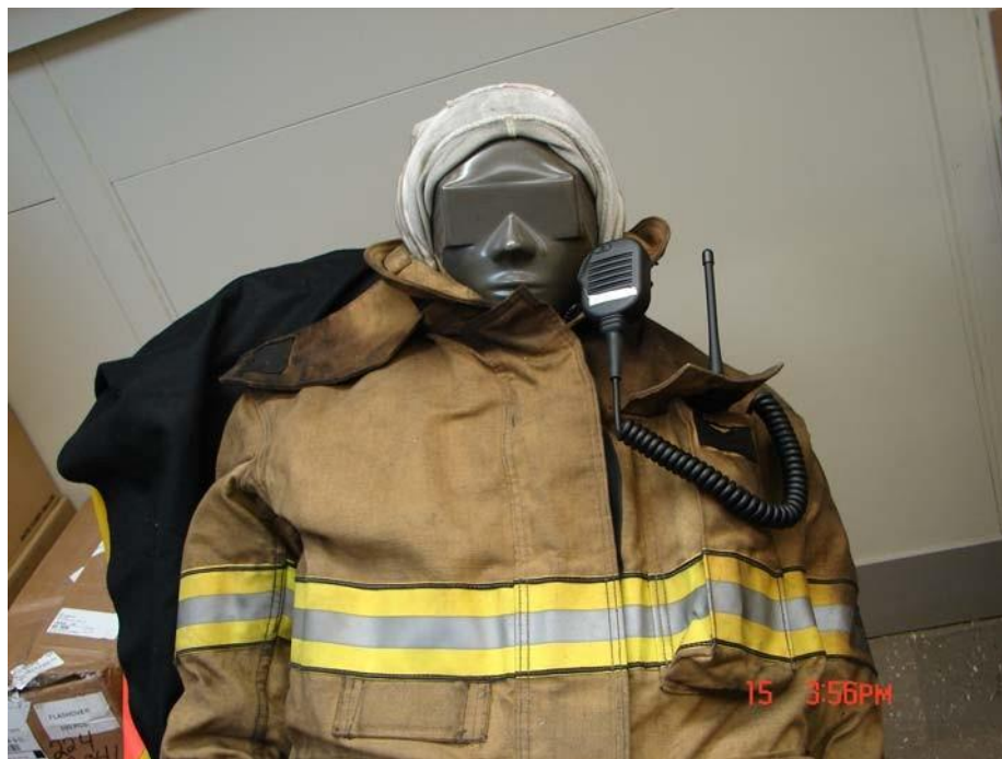
Figure 3 Radio inside turnout coat pocket with speaker/microphone 圖3 消防衣口袋內無線電（附喇叭與麥克風）
