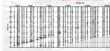
Figure 4. Shot gather of northernmost line, Line 01. Time is unredacted, and source-receiver offset is in meters. First arrival picks (red asterisks) are shown on the traces. Data have been filtered (6-8-12-48 Hz bandpass window), had automatic gain control (AGC) applied, and top- and bottom-muted (shaded areas).
